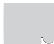
Cockbead 8 mm Overall 7mm bead 1mm flat
