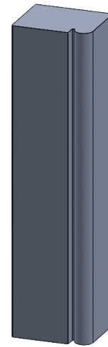
Cockbead 8 mm Overall 7mm bead 1mm flat
