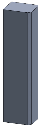
3 x 3 mm Chamfer Chamfer to external vertical edge of frame. 3 mm x 3 mm Chamfer.
